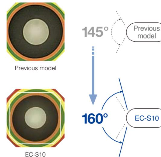
The white lines indicate the angle of view of the previous model.
